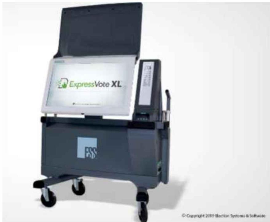
34. A voter uses the ExpressVote XL by inserting into the device a 4.25-inch wide blank card made of thermal paper.
